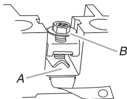
A. Insert wire under screw clamp
