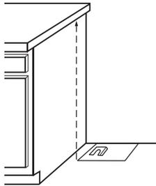
If cabinet opening is wider than that specified in the "Location Requirements" section, adjust template so range will be centered in cabinet opening.
