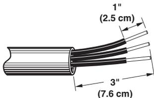
4. Allow enough slack in the wire to easily attach the wiring terminal block.
