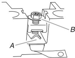
A. Insert wire under screw clamp
