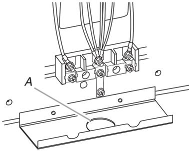
A. Remove knockout for 40- or 50-amp power cord and UL listed strain relief
